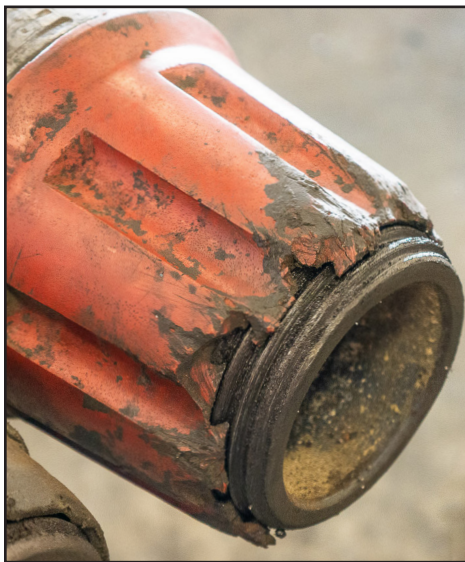
Severely damaged thread protector
