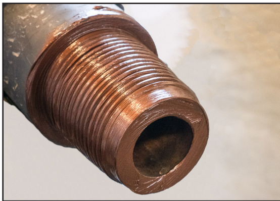
Correct application of compound
