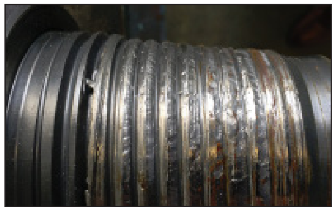
Extremely damaged TDSS sent for "repair"
