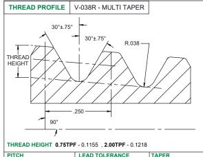
LEAD TOLERANCE 2.00 TAPER PER FT. (.0625 in/in) 0.75 TAPER PER FT. (.1667 in/in) 4 THREADS PER INCH (.250 LEAD) +.003 PER 1 INCH SEE NOTE 5
