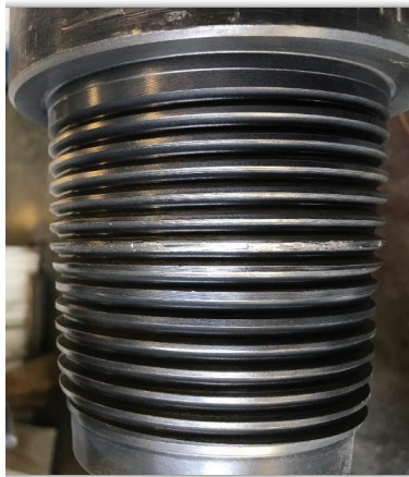
Landing Pad Wear
